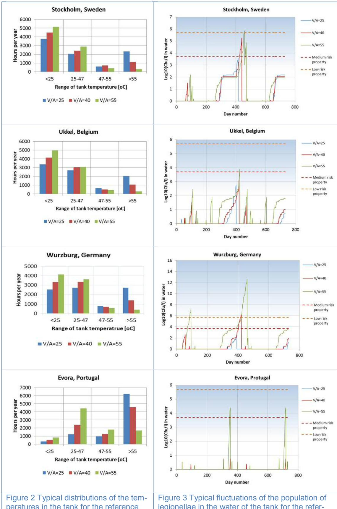
Figure 2 Typical distributions of the temperatures in the tank for the reference
